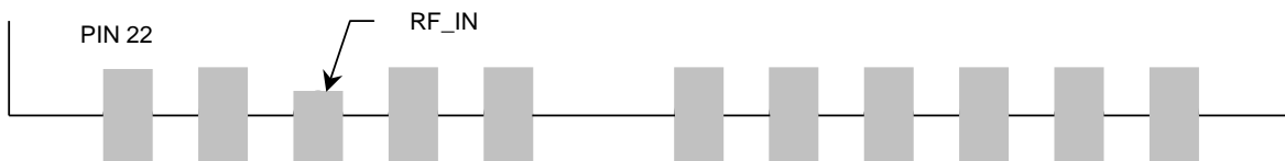
Figure 4 Solder Pad Size and Placement
